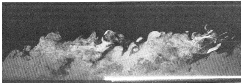
158. Turbulent boundary layer on a wall. A fog of tiny oil droplets is introduced into the laminar boundary layer on the test-section floor of a wind tunnel, and the layer then tripped to become turbulent. A vertical sheet of light
